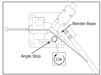
Figure 17. Using angle stop.
